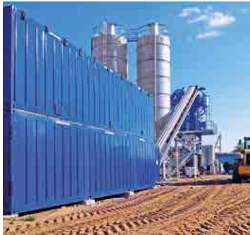
^ Semi-Mobile Batching Plant Type MCM
